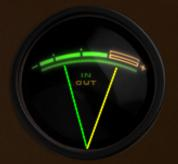
ENERGY DELTA In mathematics, 'Delta' is the measure of variation or change in a variable. Novatron's simple trick of superimposing the Input and Output meter directly on top of one another makes it extremely easy to see the change in energy and movement of a sound as a result of the processing applied. It also makes quick work of accurately matching Input and Output levels, allowing the operator to make more accurate a/b comparisons.
